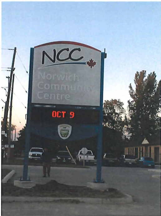
Norwich Arena Design and concept Halo lit letters with aluminum faces Mono LED Display Manufactured and installed by Banner Promotions
