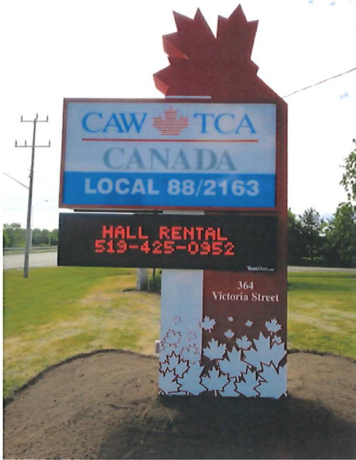
Recently replaced pylon for Unifor Local 88 Ingersoll, ON Design and concept matching colours and logo New pylon sign with existing LED Display reused Sign cabinet with lexan faces Manufactured and installed by Banner Promotions
